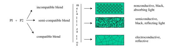
Morphology of the films, based on PI blended with P2 polymer determines physical properties of final metallized composites
